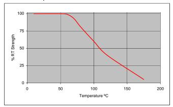
**Heat Aging** Aged 2000 hours - Tested at (22°C).
